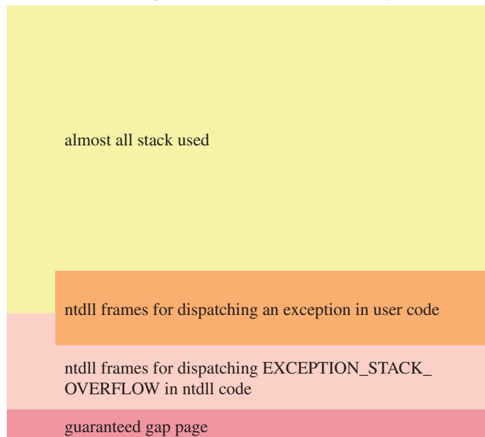
Stack during broken stack overflow delivery:
