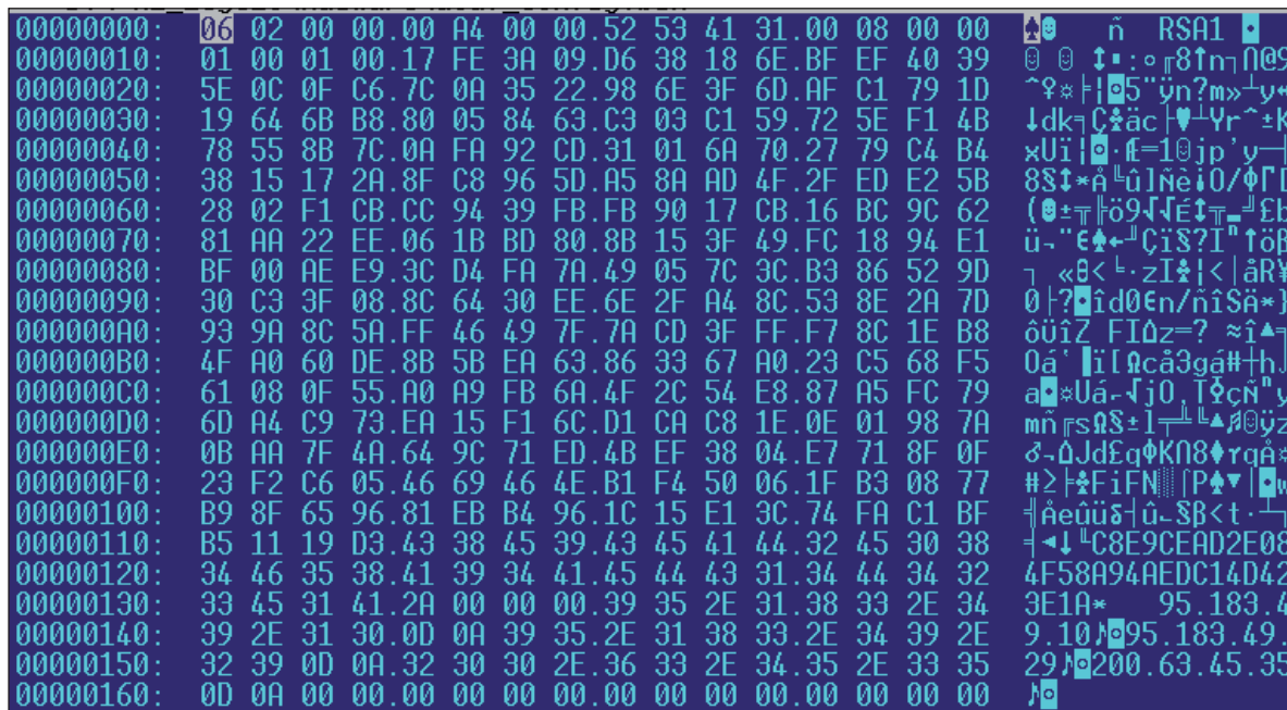
Figure 3: Decrypted configuration data contains an RSA public key to encrypt exfiltrated data, C2 IPs and unique ETag to communicate with them.
