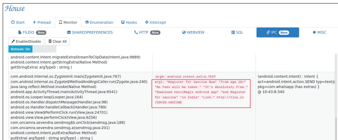
Figure 15: The Android/Oji malware sends the message to WhatsApp as an extra intent. This is detected by House.
